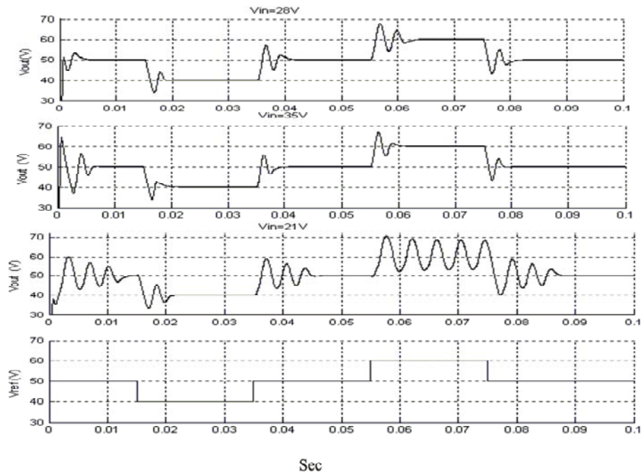
Fig.(15) : Reference voltage tracking ability
